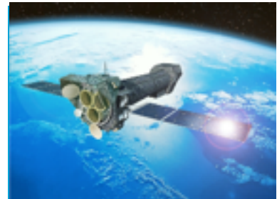
The satellite XMM Newton (X-ray Multi-Mirror) was launched by the European Space Agency in 1999. It gives a cartography of the sky between 0.1 and 12 keV.
